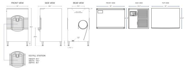
INSTALLATION NOTE: ALLOW 6" SPACE AT LEFT, BACK, AND RIGHT SIDES FOR VENTILATION AND UTILITY CONNECTION
