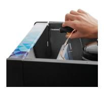
7. Re-attach the left-side end cap and top panel by replacing and attaching the previously removed screws.
