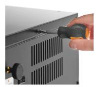
2. Unscrew the (3) screws on the back of the unit connected to the top panel.
